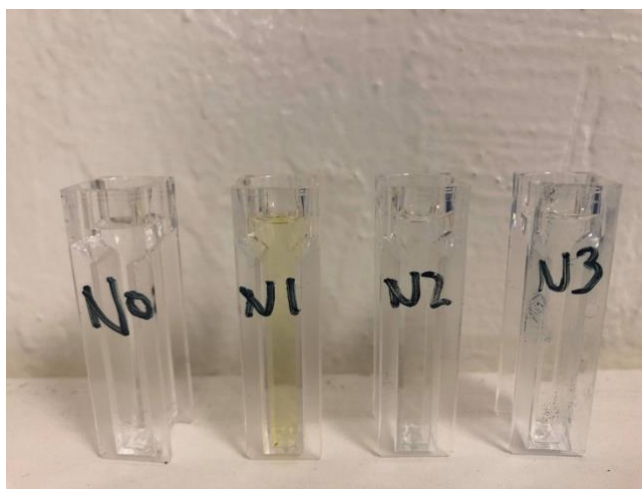
Figure 2: Picture of cuvettes, left to right: N0 — Blank, N1 — 4-nitroacetanilide and Nattokinase, N2 — 4-nitroacetanilide control, N3 — Nattokinase control.
